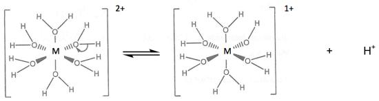
• This reaction is often referred to as **hydrolysis** or **acidity** reaction as there is a reaction with water producing an acidic solution
